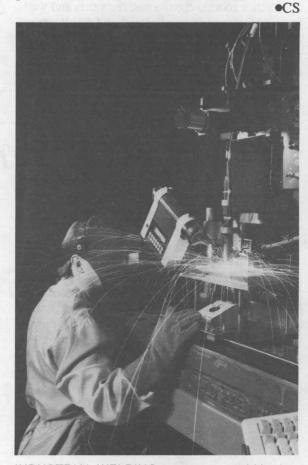
INDUSTRIAL WELDING processes could be improved by Sandia research, potentially increasing US industry's global competitiveness. Here, Rick Blum (8312) welds metal as diagnostic equipment checks the work. Sandia researchers are also working on computer simulations of welding processes. (Photo by Cary Chin, 8275)
